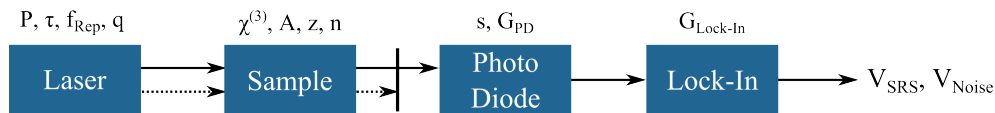
Figure 3.5: SRS principle and most influencing parameters on the signal voltage and background noise
